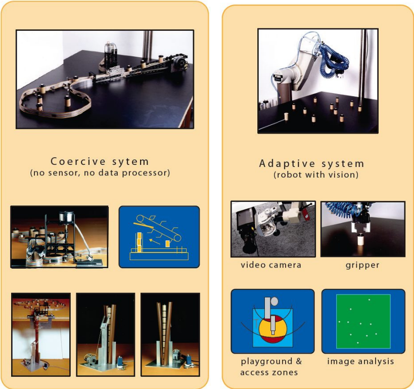
Figure 22. Experimental implementations. Left: coercive system (no sensor). Right: adaptive system (robot with vision).
