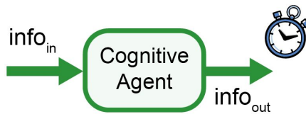
Fig. 4 – Behavioral model . A CS is mainly characterized, in MCS theory, by incoming information, ( I_{in} ), and, respectively, outgoing information, ( I_{out} ). In essence, a CS has the capability of generating the relevant information, ( I_{out} ). Time is sometimes also a significant dimension.
