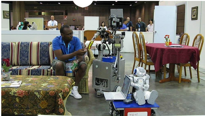
Fig.17 Nono, a humanoid of Nao type (lower right) mediates between humans and other machines. OP-Y is the platform on which Nono is installed; RH-Y is the robot who brought drinks and snacks. http://rahe.populus.ch .
